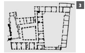
Figure 3. Plan of the early-modern convent of Norbertine Nuns in Imbramowice, with the locations of surviving fragments of fourteenth- and fifteenth-century walls of the church marked in green. Drawing after Andrzej Krupiński. → see p. 71
