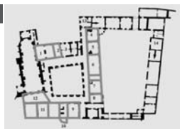
Figure 4. Plan of the early-modern convent of Norbertine Nuns in Imbramowice, with the interiors that follow the mediaeval layout marked in green. 1. Oratory connected with the sacristy, with vestry upstairs; 2. Cloister gate; 3. Parlatoria; 4. Kitchen, with the bath-house upstairs; 5. Chamber; 6. Refectory with chambers upstairs; 7. Chamber; 8. Cellar; 9. Infirmary, with monastic cells upstairs; 10. Entrance to the garden; 11. Room for secular maidens and novice nuns; 12. Chapel; 13. Auxiliary section: pantry and outbuildings; 14. Auxiliary section: granary, pantry, laundry room, bakery. Drawing after Andrzej Krupiński → see p. 73
